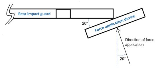
Load application. Apply the load in a direction that is perpendicular to the front surface of the load application device while guiding the device to prevent rotation. The loading rate should meet the CMVSS 223 criteria (section 5.3.1) and be applied until displacement of the force application device has reached 125 mm. The force should then be reduced until the guard no longer resists the force application device.
